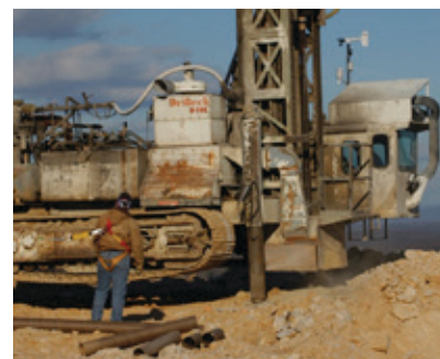
Vehicle-mounted drilling rig using water on the drill bit. The enclosed operator's cab is on the right.
